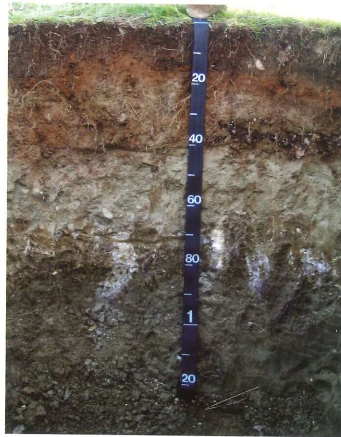
This profile from North America shows a stratified soil that has developed on volcanic material (ash and ejecta). The different colours reflect the weathering of minerals (predominantly iron and aluminium oxides) and can contain significant amounts of volcanic glass. The uppermost 15 cm shows a dark, organic-rich horizon. Such soils are typically very fertile and can usually support intensive cropping or forests. (EM)
