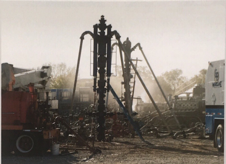
Fracking is the controversial process of freeing trapped gas by drilling and pumping in a mixture of water, sand and chemicals. Photo © www_ukberri_net.
