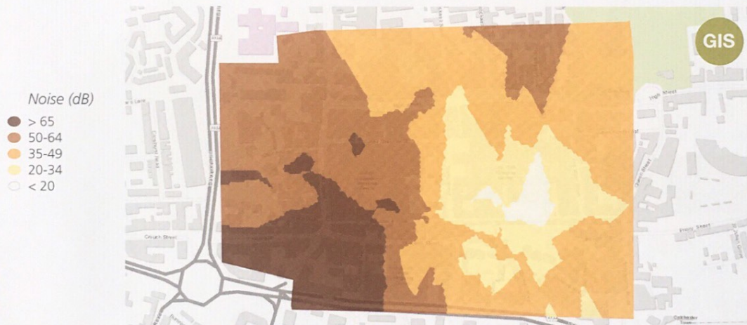
6.6 Using analysis functions in ArcGIS Online to interpolate sound levels in Colchester town centre © Esri UK 2017
