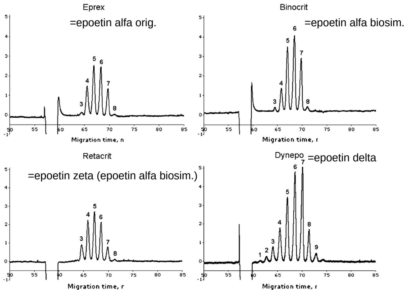
Fig. 3 CE-UV analysis of the four EPO products.
