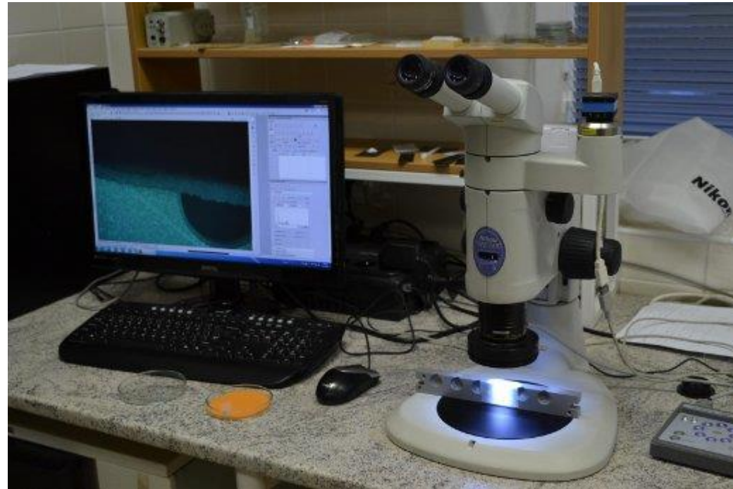
Image Analysis NIS a LECO with Optical microscope and Stereo microscope Nikon
