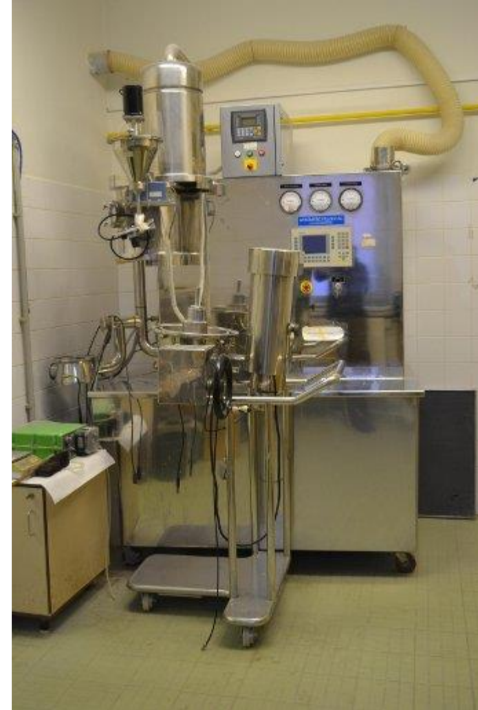
Multi Roto Processor Aeromatic (drying, granulation and coating – top, tangential spraying and wurster, rotoagglomeration)
