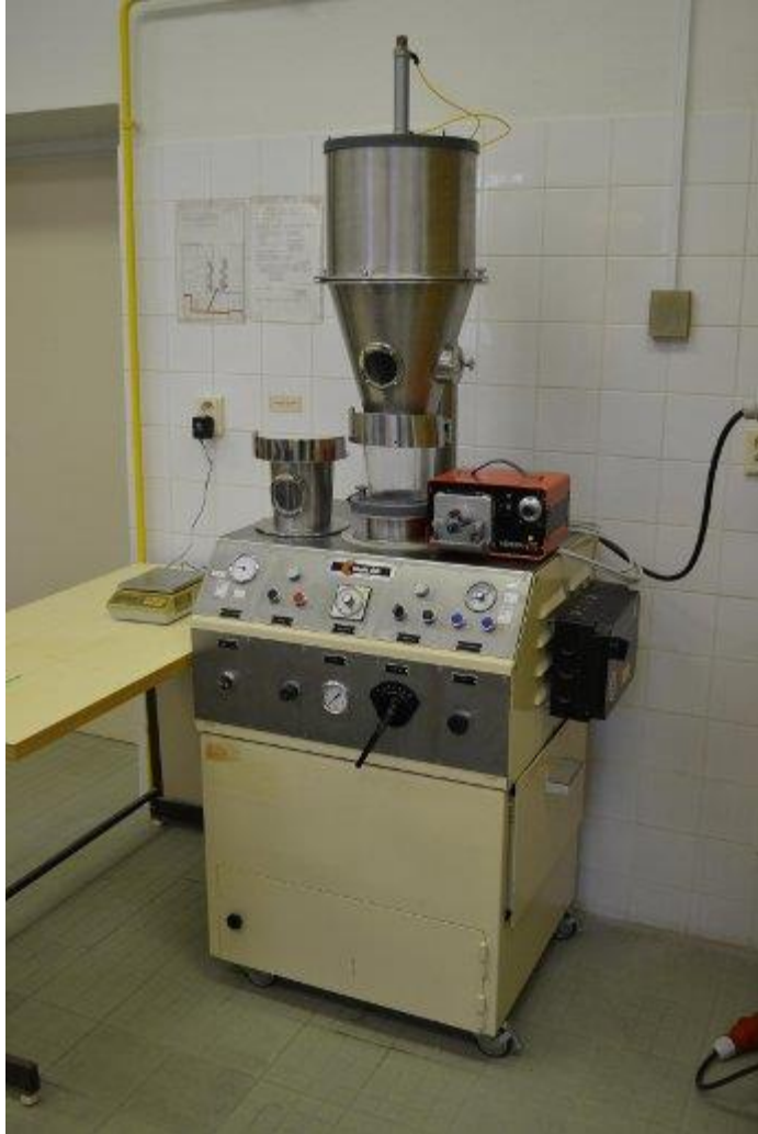
Laboratory Fluid Bed Processor Uniglatt (drying, granulation and coating - top spraying and wurster)
