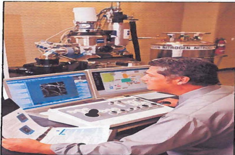
JULIE KNIGHT/THE BUSINESS JOURNAL Christopher Kopley, Ph.D., associate professor at the Joint School of Nanoscience and Nanoengineering, demonstrates use of the Zeiss helium ion microscope.
