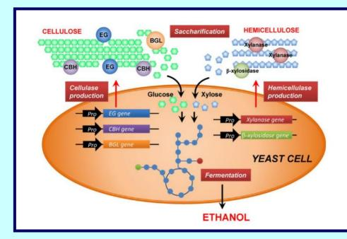
Recombinant yeast cells developed for CBP. The CBP cells have the capability to produce sufficient cellulases (EG, CBH and BGL) and hemicellulases (xylanase and  $\beta$ -xylosidase) for hydrolysis of biomass and efficient ethanol production from both glucose and xylose.
