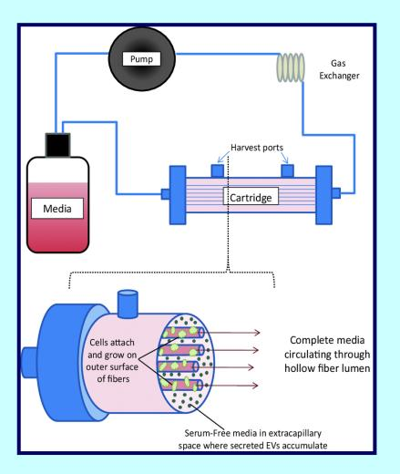
A three-dimensional system containing hollow tubes = semi-permeable capillary membranes assembled in parallel rows usually located in a carbonate tube.
