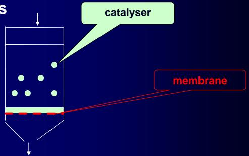
Microencapsulation – closing of a bio catalyser by a membrane into micro-capsules  $\rightarrow$  forming of emulsion
