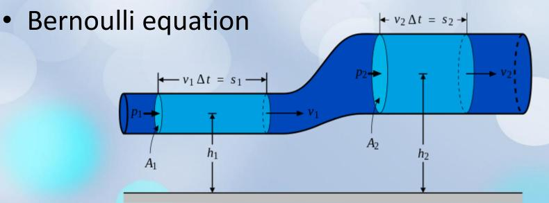
In the place with a larger cross-section the flowing liquid has higher pressure, but lower speed, in a place with a smaller cross-sectional area has a smaller pressure but greater speed
