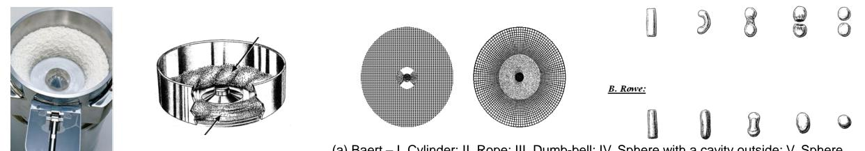
(a) Baert – I. Cylinder; II. Rope; III. Dumb-bell; IV. Sphere with a cavity outside; V. Sphere.
