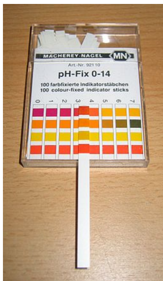
Figure 6.2 Plastic box of pH indicator paper. A single pH paper strip with four colored squares sits on top of the box. By Michael Krahe - CC BY-SA 3.0, https://en.wikipedia.org/wiki/PH_indicator#/media/File:PH_indicator_paper.jpg ( https://en.wikipedia.org/wiki/PH_indicator#/media/File:PH_indicator_paper.jpg ).
