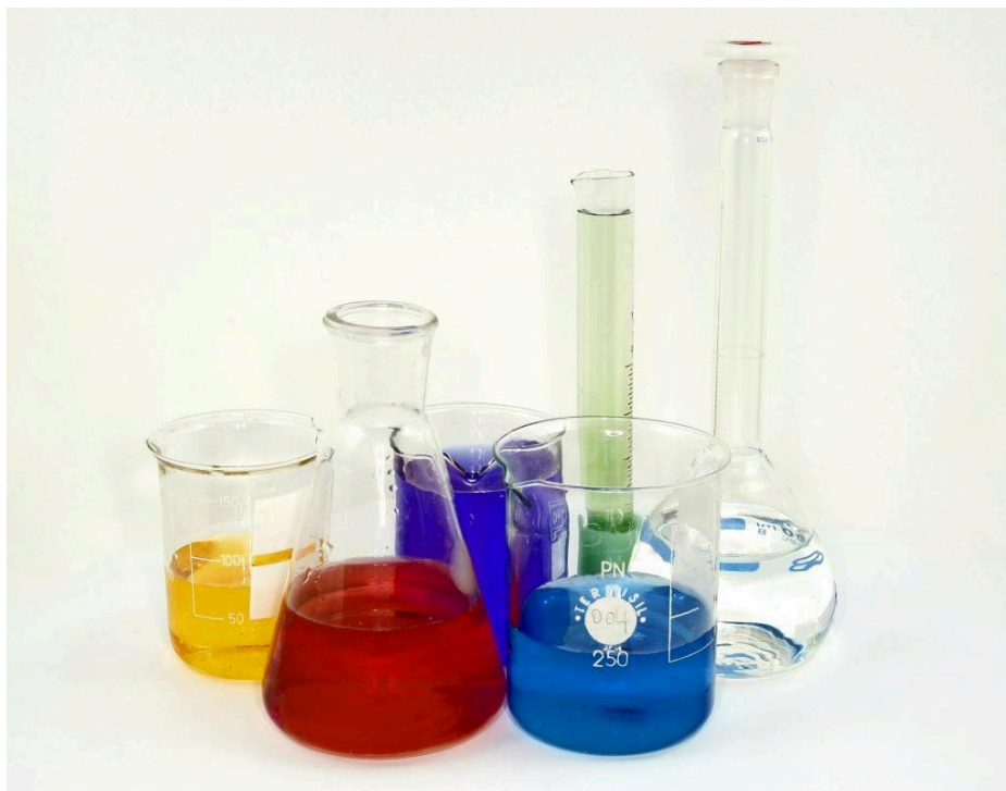
Figure 6.8 Various types of glassware; beakers, Erlenmeyer flask, graduated cylinder, and volumetric flask. Image credit: https://upload.wikimedia.org/wikipedia/commons/ffc/Lab_glassware.jpg ( https://upload.wikimedia.org/wikipedia/commons/ffc/Lab_glassware.jpg )
