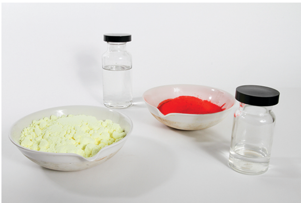
Figure 5.6 Each sample contains 6.02 \times 10^{23} molecules or formula units—1.00 mol of the compound or element. Clock-wise from the upper left: 130.2 g of C_8H_{17}OH (1-octanol, formula mass 130.2 amu), 454.4 g of HgI_2 (mercury(II) iodide, formula mass 454.4 amu), 32.0 g of CH_3OH (methanol, formula mass 32.0 amu) and 256.5 g of S_8 (sulfur, formula mass 256.5 amu). (credit: Sahar Atwa)
