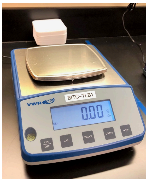
Figure 6.5 VWR top loading electronic balance. Photo credit: Jeremy Garza, Austin Community College.
