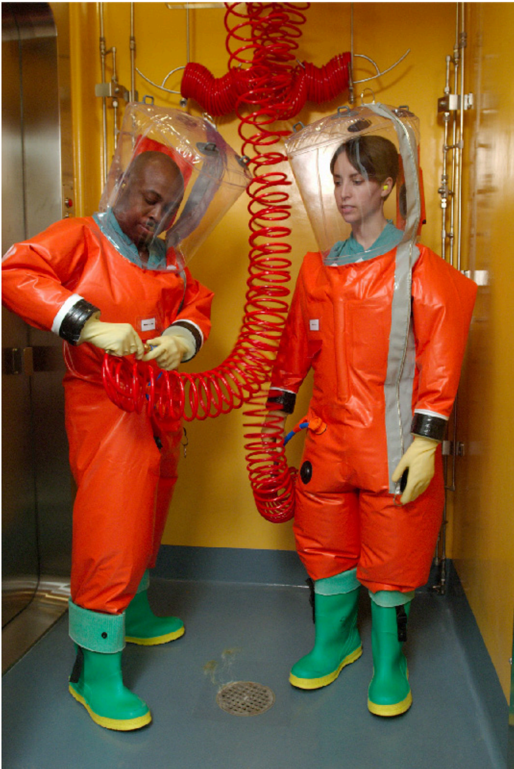
Figure 11.2 A protective suit like this one is an additional precaution for those who work in BSL-4 laboratories. This suit has its own air supply and maintains a positive pressure relative to the outside, so that if a leak occurs, air will flow out of the suit, not into it from the laboratory. (Credit: James Gathany, CDC, public domain)
