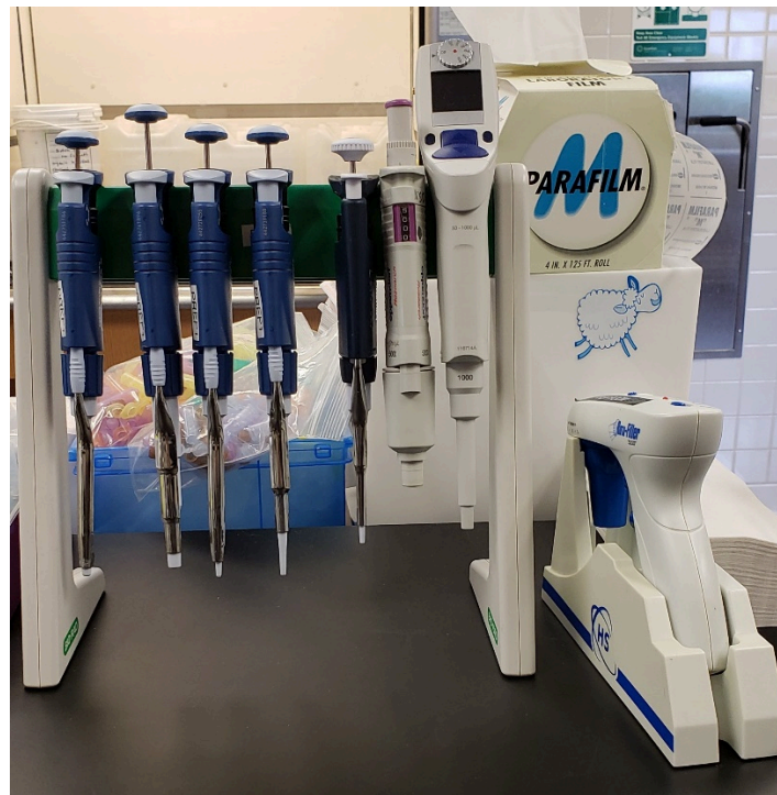
Figure 6.9 Various micropipetting devices. From left to right: Set of 6 micropipettes measuring capacities from 2 microliters to 5 mL; 1 mL ergonomic digital micropipette; electronic pipet-aid (to draw liquid into serological pipet). Image Credit: Jack O'Grady, Austin Community College
