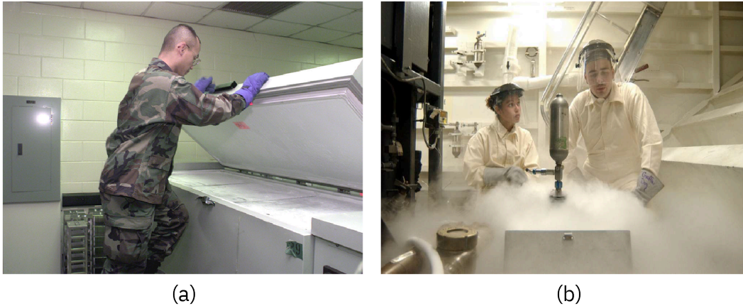
Figure 11.10 Cultures and other medical specimens can be stored for long periods at ultra-low temperatures. (a) An ultra-low freezer maintains temperatures at or below -70^{\circ}\text{C} . (b) Two people stand in a room with a large nitrogen storage unit emitting a large amount of fog. (credit a: modification of work by “Expert Infantry”/Flickr; credit b: Credit: US Navy; Public Domain.)
