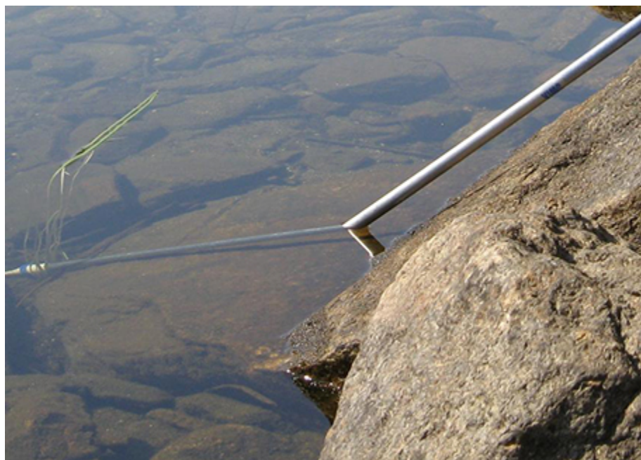
Figure 9.5 This straight pole appears to bend at an angle as it enters the water. This optical illusion is due to the large difference between the refractive indices of air and water.
