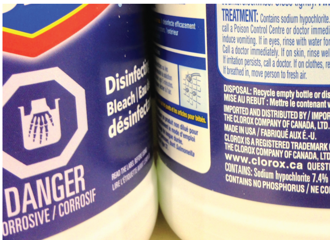
Figure 5.14 Liquid bleach is an aqueous solution of sodium hypochlorite (NaOCl). This brand has a concentration of 7.4% NaOCl by mass.
