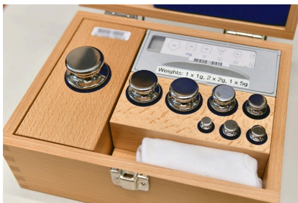
Figure 6.11 Electronic balance calibration weight set. Image credit: Dean Calma / IAEA https://www.flickr.com/photos/iaea_imagebank/40785322521 ( https://www.flickr.com/photos/iaea_imagebank/40785322521 )
