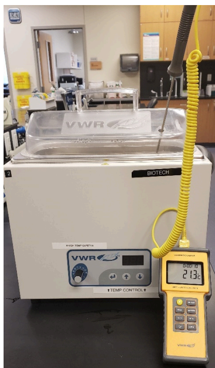
Figure 6.12 Calibrated digital thermometer can be used to accurately measure temperatures. In this figure, a (yellow) calibrated digital thermometer is being used to measure the temperature of a water bath. Image credit: Jack O'Grady, Austin Community College.
