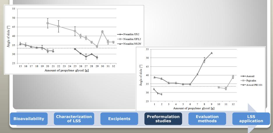
DETERMINING of the FLOW RETENTION POTENTIAL of carriers (MCC, Fujicalin, Neusilin US2 a NS2N) and coating materials (Aerosil 200 a Neusilin UFL2) for PG
