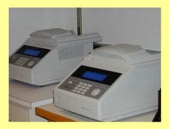
Termocyclers quickly change temperature in reaction blocks between the three temperatures of the PCR cycle
