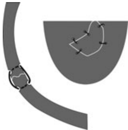
Fig. 1 Representation of the earliest type of repair: drilling holes and tying the sherds together using rope or leather.
