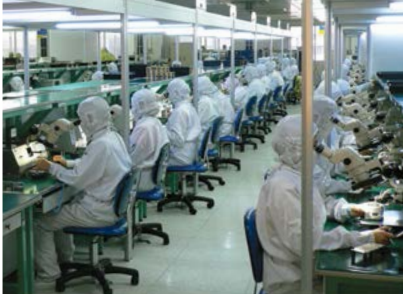
Workers assembling and testing fiber optic systems. Photo: Steve Jurvetson
