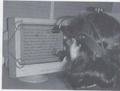
Fig. 2.31 The EyeLink I 250 Hz system, with head-mounted camera and LED markers around the stimulus to define the coordinate system. For clarity, two of the LEDs have been circled. Picture used with kind permission from SR Research.
