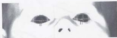
(a) Eye-video from participant aged 48 days successfully tracked with dark-pupil remote eye-tracker.
