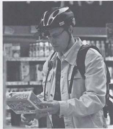
(b) SMI HED-mobile system with recording computer in rucksack (from 2008). Photo used courtesy of Gunnar Menander and Petra Francke.
