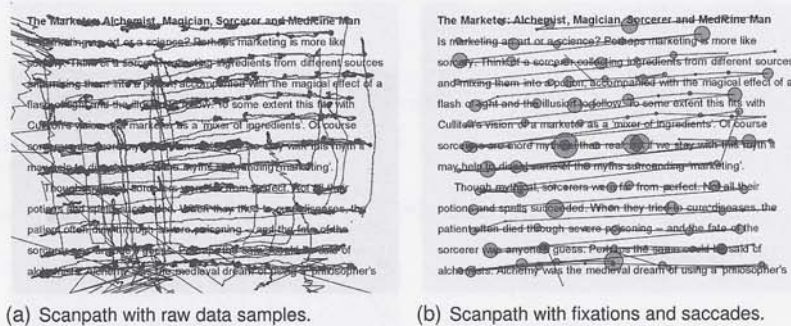
Fig. 5.3 Data recorded at 1250 Hz with a tower-mounted eye-tracker. Fixations were calculated with the commercial software BeGaze 2.1, applying a velocity-based analysis and default settings with a peak velocity threshold of 75^\circ/\text{s} . Note that parsing the data using this algorithm omits some of the grouped samples of 'blobs' which from manual inspection seem to be valid fixations.
