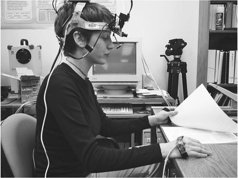
FIGURE 1.9 The associate training the computational model is wearing ASL eye tracker, CCD camera, microphone, and position sensors. The computational model thus shares multisensory information like a human language learner. This allows the association of coincident signals in different modalities. (From Yu, Ballard, and Aslin 2005, by permission)
