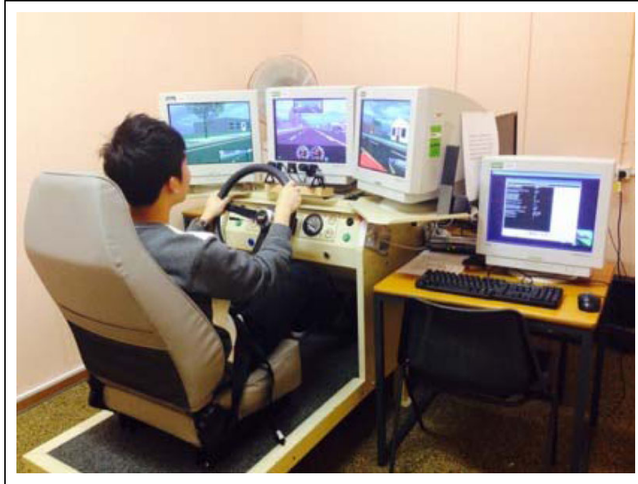
Figure 1. STISIM Drive 400 driving simulator.
