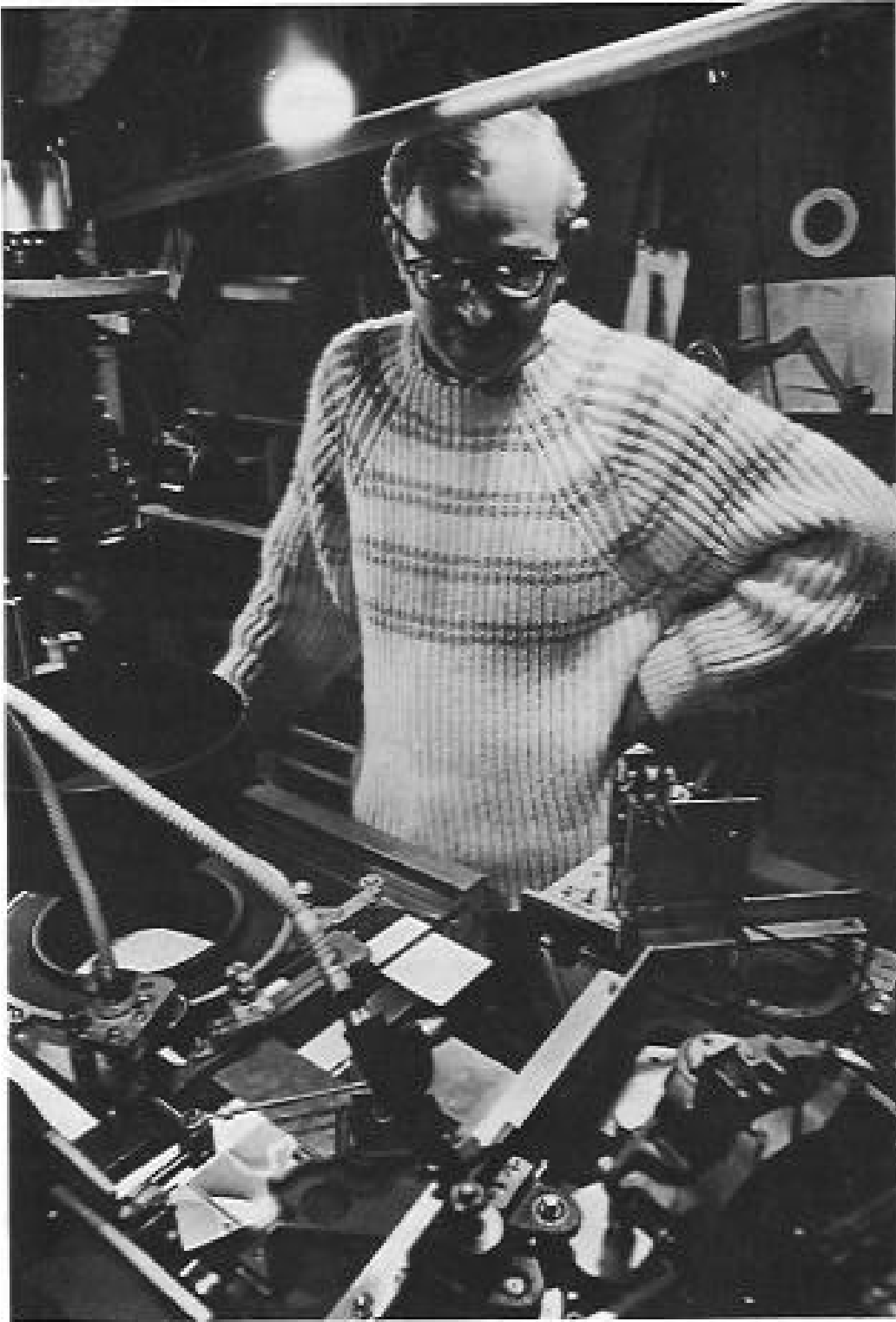
John Whitney working with his mechanical analogue computer. Photo: Charles Eames.
