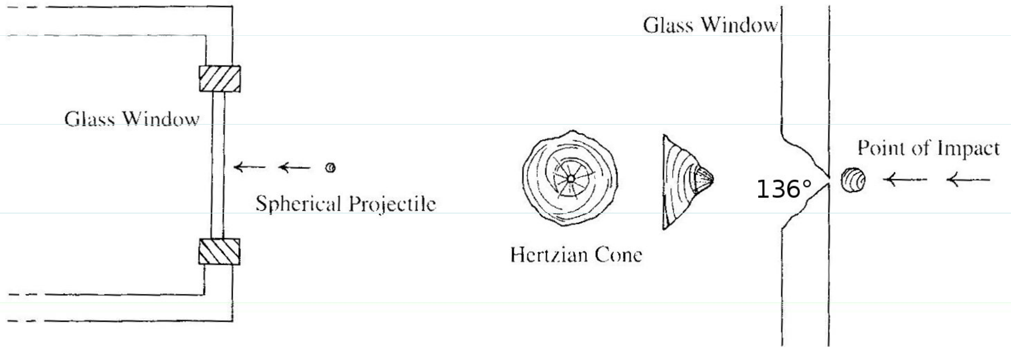
FIGURE 2.12 Schematic illustration of spherical projectile impacting a pane of glass at a 90 degree angle to produce a Hertzian cone.
