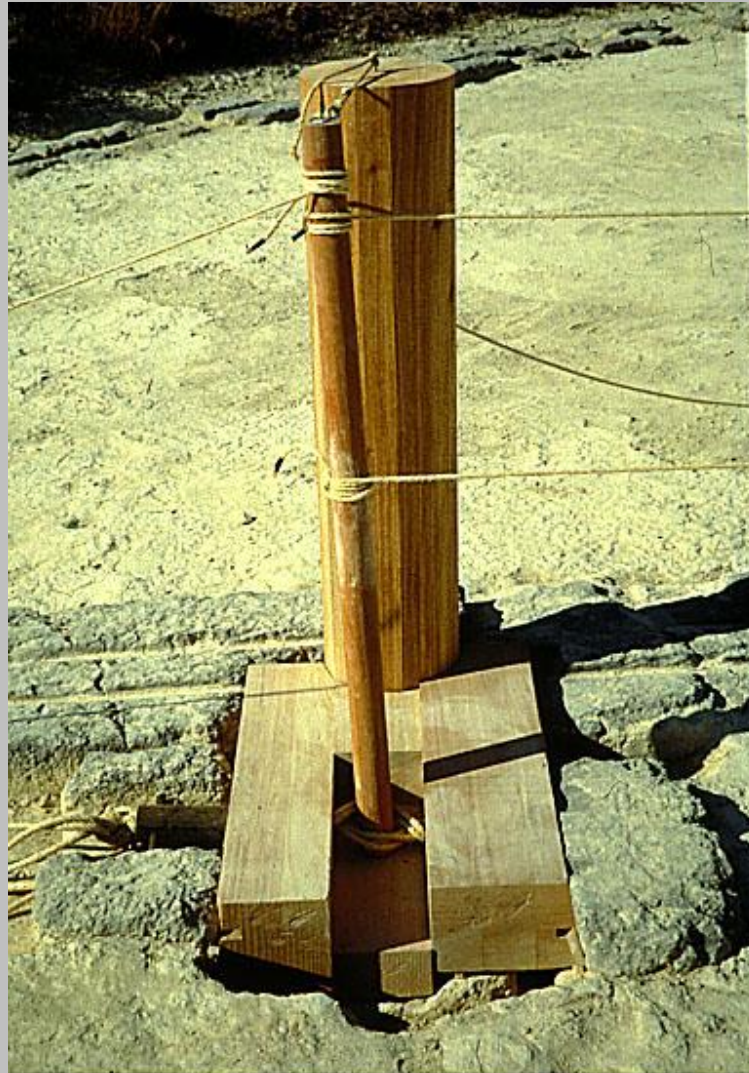
103) Detail of actual reconstruction of Nemea hysplex showing twisted ropes that produce torsion energy to drive the machine.
