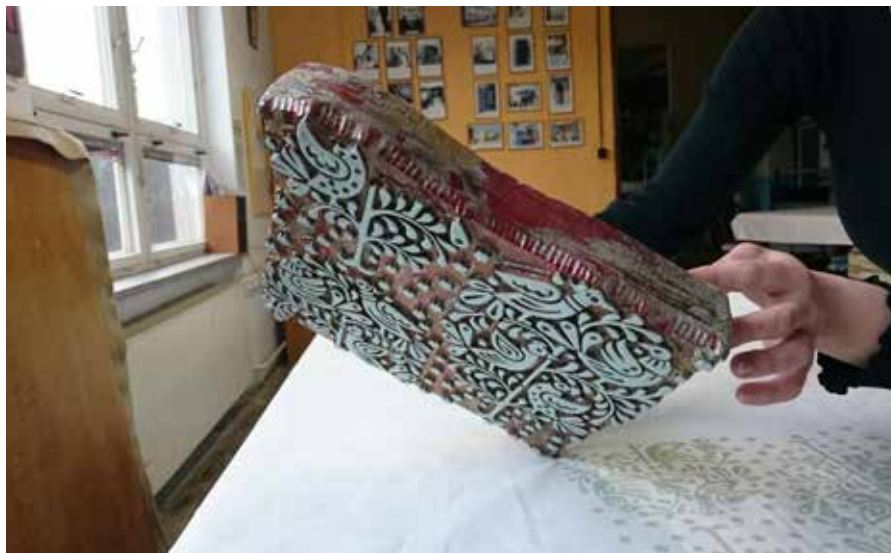
Linen printing using a carved block dipped in the dye-resist paste ( pop ). The Joch workshop in Strážnice. Photo: Martin Sitek, National Institute of Folk Culture, 2017
