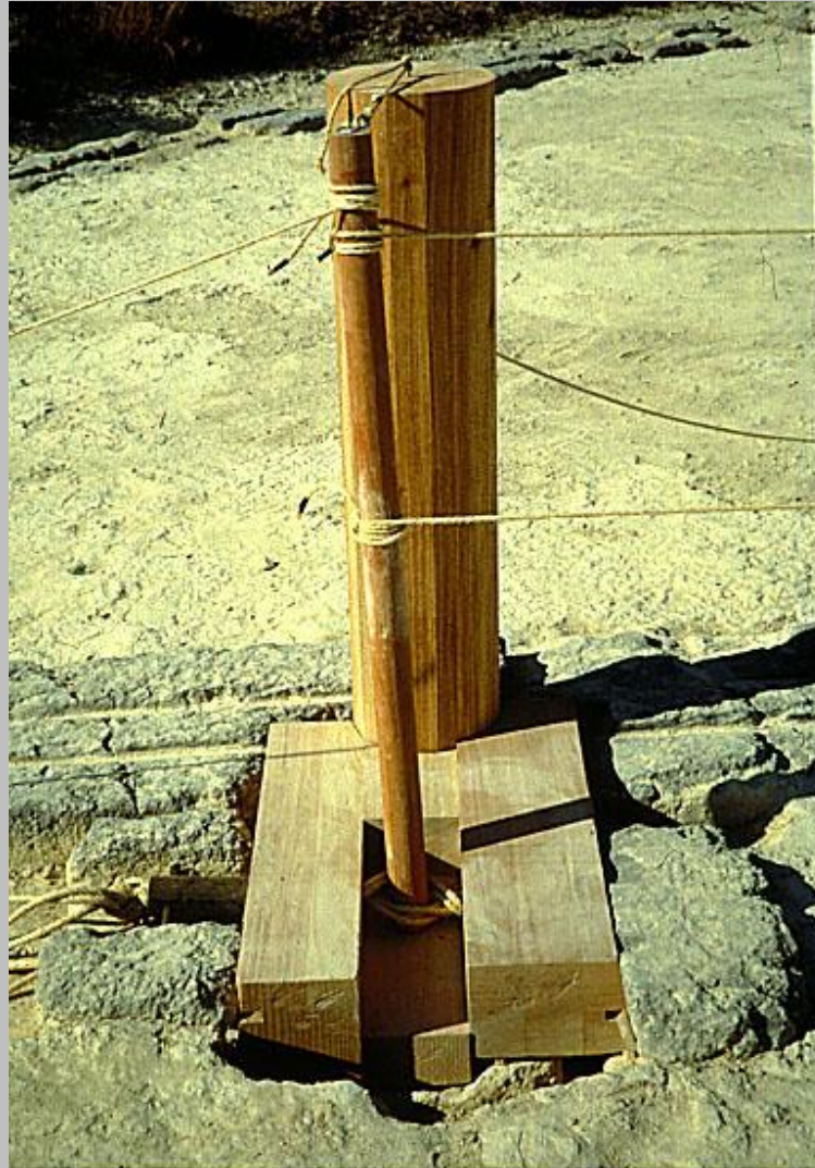
103) Detail of actual reconstruction of Nemea husplex showing twisted ropes that produce torsion energy to drive the machine.
