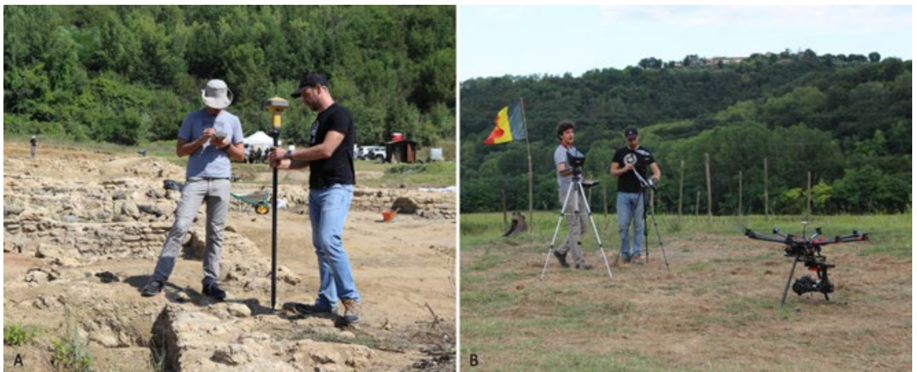
Fig. 2. A) registration of topographic GCP with a differential GPS; B) ground control station with 2 remote controllers (for UAV and Gimbal) and 2 monitors connected in streaming with 2 video cameras. The first camera is mounted on the chasis to drive the UAV, and the second one is located on the gimbal to control camera movements.
