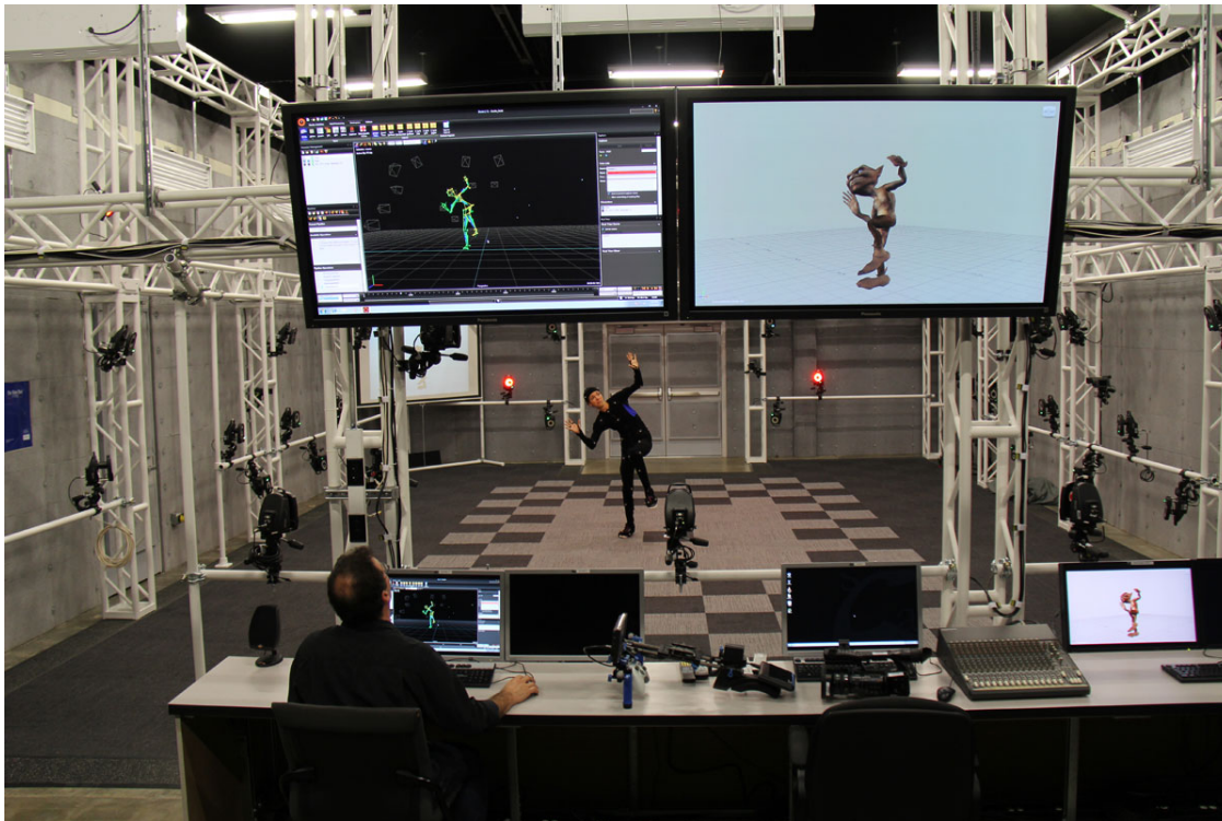
9.3. Typical use of motion capture in cinema and video games: the movements of an actor are captured and used to drive an animated character.
