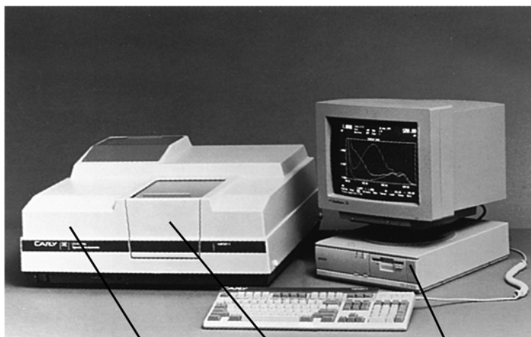
Source, monochromator, detector Sample compartment Display and controls
