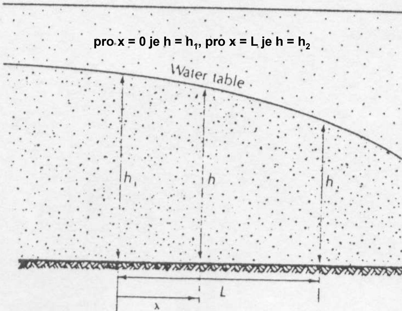
$$h^2 = h_1^2 - \frac{(h_1^2 - h_2^2)x}{L} + \frac{w}{k}(L-x)x$$
