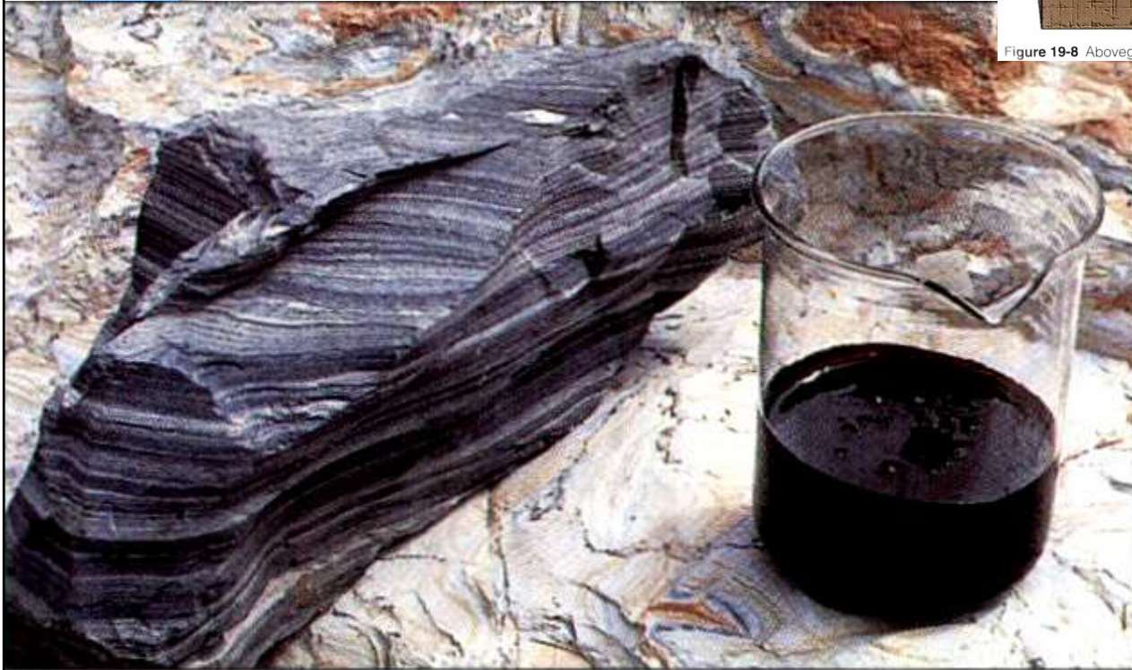
Figure 19-7 Oil shale and the shale oil extracted from it. Big U.S. oil shale projects have been canceled because of excessive cost. (U.S. Department of Energy)
