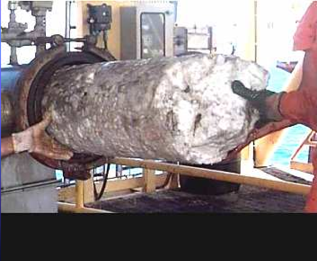
Figure-2 A large gas hydrate plug formed in a subsea hydrocarbon pipeline. Picture from Petrobras (Brazil).
