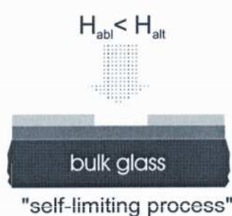
Figure 6. Schematic presentation of the assumed ablation characteristics of different layers and the consequences for the ablation process ( H_{abl} = ablation threshold, H_{alt} = alteration threshold).
