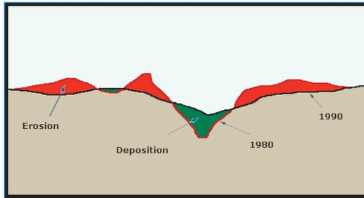
The Cut/Fill function performs the surveying for you, identifying the areas that have been eroded, the areas of deposition, and the areas of no change. It also calculates the volume of surface material that has been cut or filled in each area.
