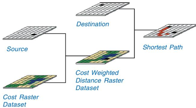
By applying a global function to a weighted—cost—surface, you can determine the cost of moving from a destination cell—the location where you wish to end the road—to the nearest source cell. To take this one step further, the shortest path over a cost surface can be calculated over a nonnetworked surface from a source cell to a destination cell. In all the global calculations, knowledge of the entire surface is necessary to return the solution.
