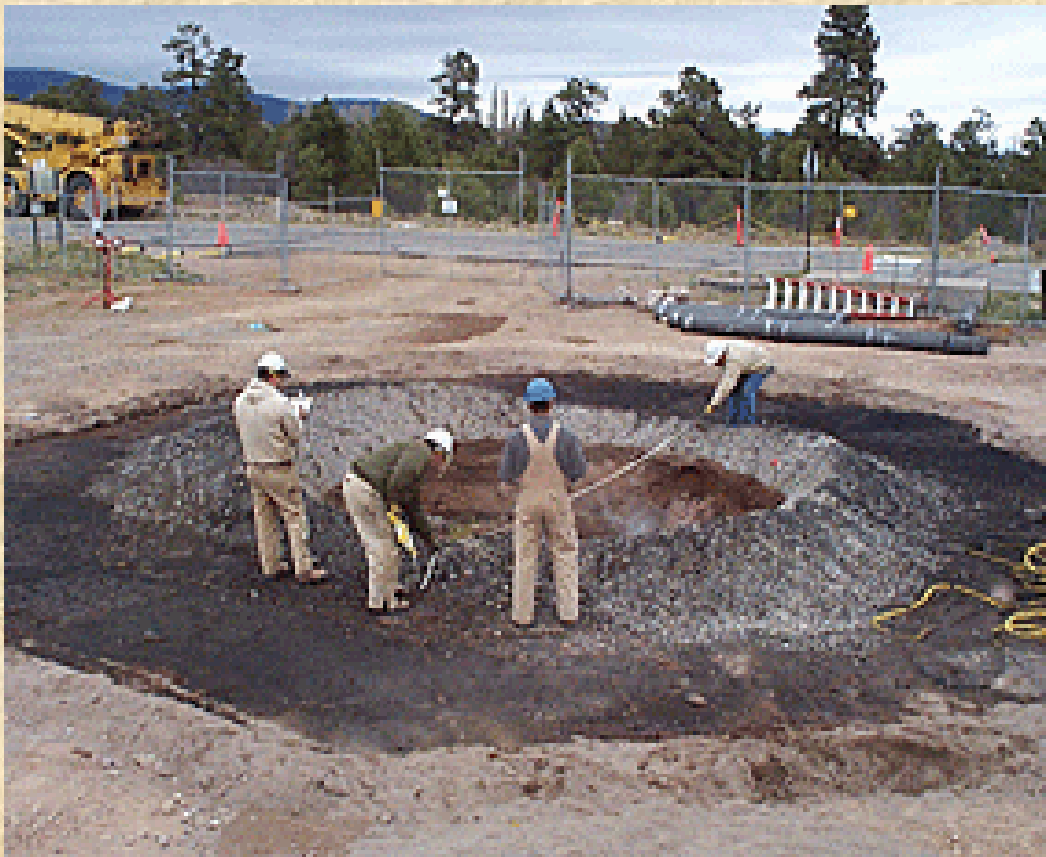
Measuring the monolith created by the planar melt cold test at Los Alamos National Laboratory.
