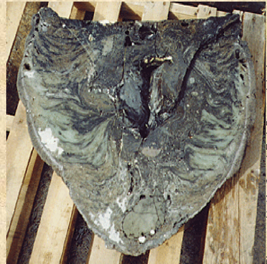
Cross section of a vitrified monolith from the Savannah River Site demonstration.
