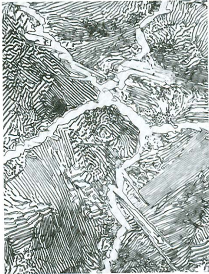
FIGURE 9.31 Photomicrograph of a 1.4 wt% C steel having a microstructure consisting of a white proeutectoid cementite network surrounding the pearlite colonies. 1000 \times . (Copyright 1971 by United States Steel Corporation.)
