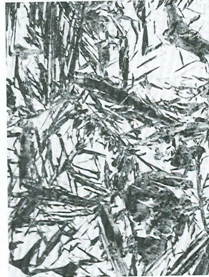
FIGURE 10.13 Photomicrograph showing the lenticular or plate martensitic microstructure. The needle-shaped grains are the martensite phase, and the white regions are austenite that failed to transform during the rapid quench. 1220X. (Photomicrograph courtesy of United States Steel Corporation.)
