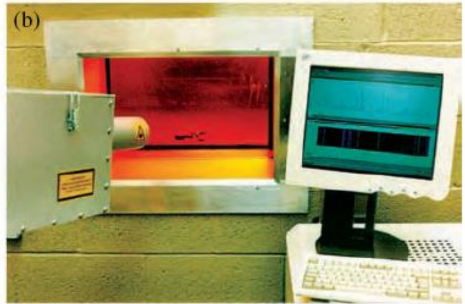
Plate 13 (a) Schematic showing the deployment of the remote LIBS instrument to monitor surface contamination. (b) Laser beam of the instrument being directed through the lead glass shield window (Applied Photonics, 2004a. Courtesy of Applied Photonics, Ltd) (see Figure 7.7)
