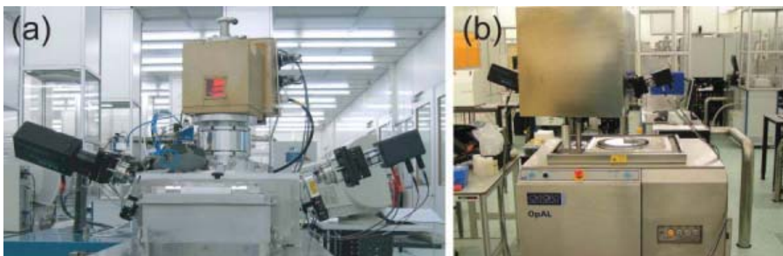
Figure 2. Photograph of a J.A. Woollam, Inc., M2000 spectroscopic ellipsometers fitted on (a) the FlexAL™ and (b) the OpAL™ reactors of Oxford Instruments [11,12]. Both commercial reactors are installed in the clean room facility of the Eindhoven University of Technology.
