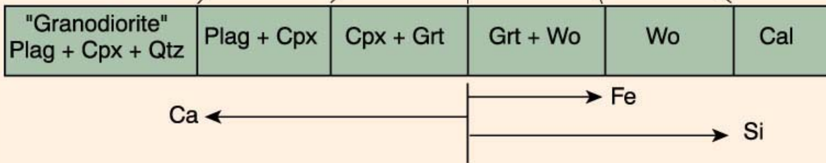
Zonation in an experimental skarn formed at the contact between granodiorite and limestone at 600°C, P_{fluid} = 0.1 GPa ( X_{CO_2} = 0.07 ). After Zharikov, V.A. and G.P. Zاراisky (1991) Experimental modeling of wall-rock metasomatism. In L. L Perchuck (ed.), Progress in Metamorphic and Magmatic Petrology. A Memorial Volume in Honor of D. S. Korzhinskii . Cambridge University Press. Cambridge, pp. 197-245. Photo courtesy G. Zاراisky. Winter (2001) An Introduction to Igneous and Metamorphic Petrology . Prentice Hall.
