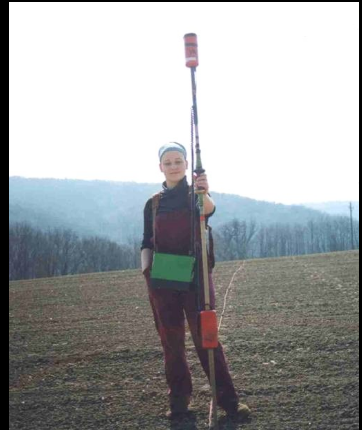
Proton magnetometer PMG-1 fa in gradient mode, Geofyzika Brno
