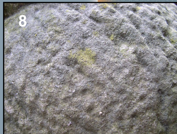
Figs 3-8. Kozia brána Cemetery: Figs. 3-4. Landform of the Kozia brána Cemetery; Fig. 3. The southern part of the cemetery; Fig. 4. Near the entrance; Fig. 5. Litava limestone; Fig. 6. Travertine; Fig. 7. Sandstone with calcareous cement; Fig. 8. Calcarenite.
