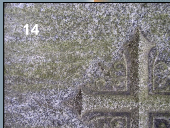
Figs 9-14. Kozia brána Cemetery: Fig. 9. Black dolerite – smooth surface; Fig. 10. Black dolerite – ragged surface; Fig. 11. Neogene calcarenite; Fig. 12. Brick; Fig. 13. Rhyolite; Fig. 14. Granodiorite.
