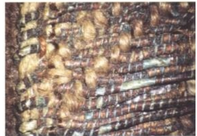
Fig. 6 Gew 582: Copper strip wound around a linen core
