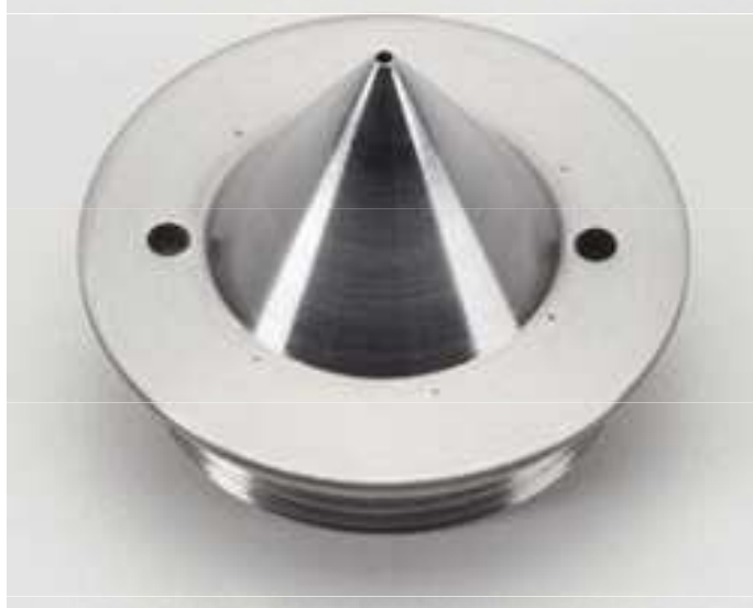
Obr. 9 Apertury rozhraní: Sampling cone a Skimmer cone .
