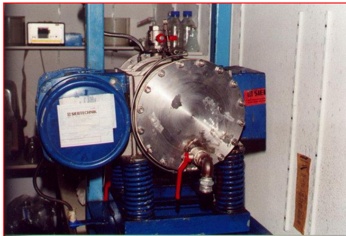
Sketch and photo of the DMCR vibratory mill (mobile design)
