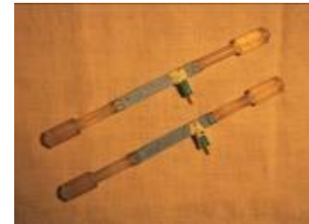
Capillary isotachopheresis modules made by Low temperature Cofired Ceramics
