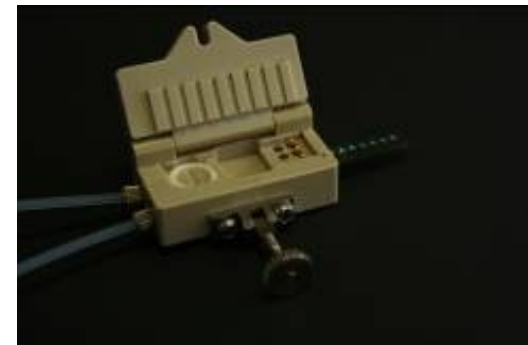
Microfluidic cell for sensors AC1 with hydraulic connectors
