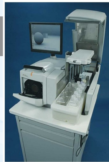
The 454 Life Sciences GS FLX sequencing system is used in many metagenomics projects.
