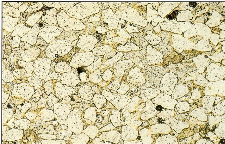
109 Quartz Arenite in plane-polarized light. Locality: New Red Sandstone, Permo-Trias, England (x 47).
