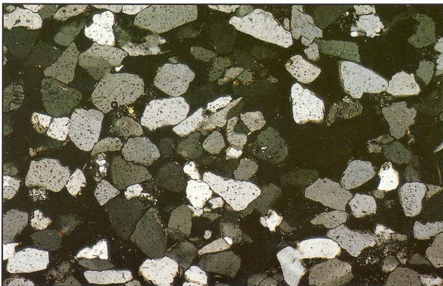
110 Quartz Arenite with crossed polars. Locality: New Red Sandstone, Permo-Trias, England (x 47).
