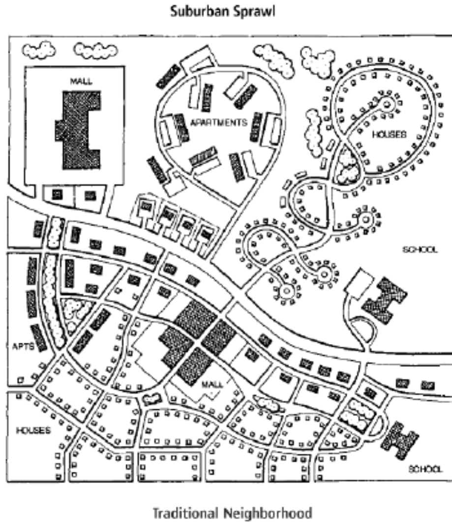
■ FIGURE 1-3 Schematic comparison of street networks and land use in sprawl (upper part of diagram) and traditional neighborhood (lower part of diagram)
