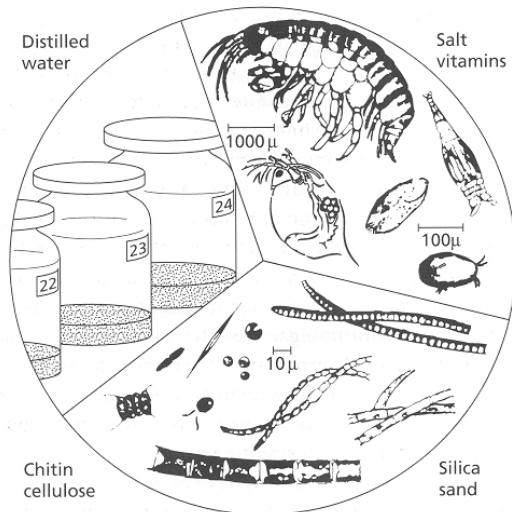
Fig. 5.2 Components of a standardized aquatic microcosm.
