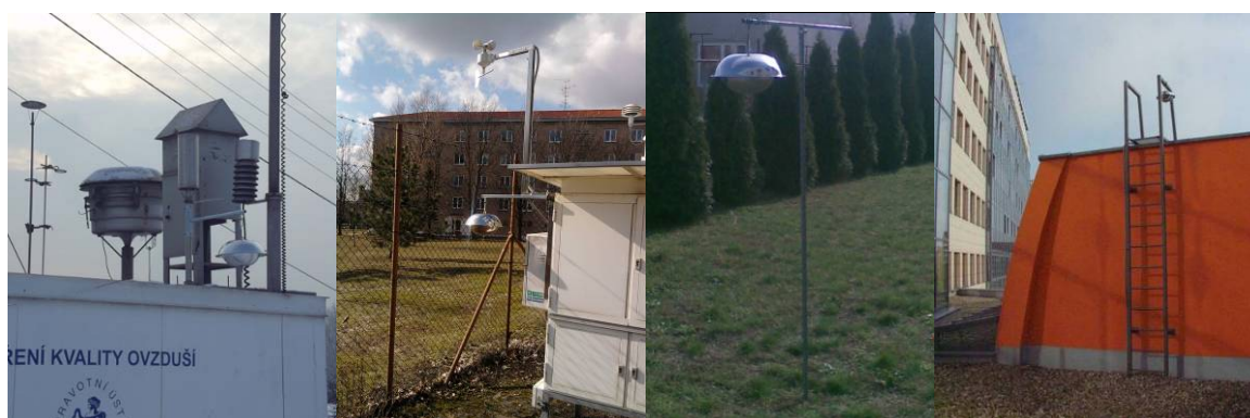
Placement of passive air sampler.
