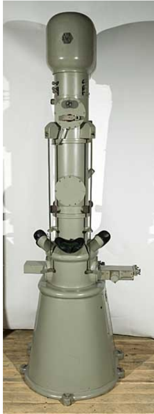
First commercial EM, 1937 Metropolitan-Vickers EM1 (EM2 shown)
